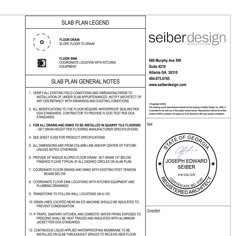
FINISH. MEMBRANE TO BE EXTENDED 6" VERTICALLY ONTO SUBSTRATE OF ALL WALLS, AND TO BE COORDINATED WITH DRAIN INSTALLATIONS PER MANUFACTURER'S INSTRUCTIONS & RECOMMENDATIONS.
